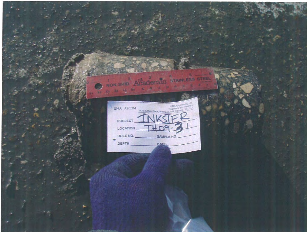
Photo 21: Core sample from TH-09-31
