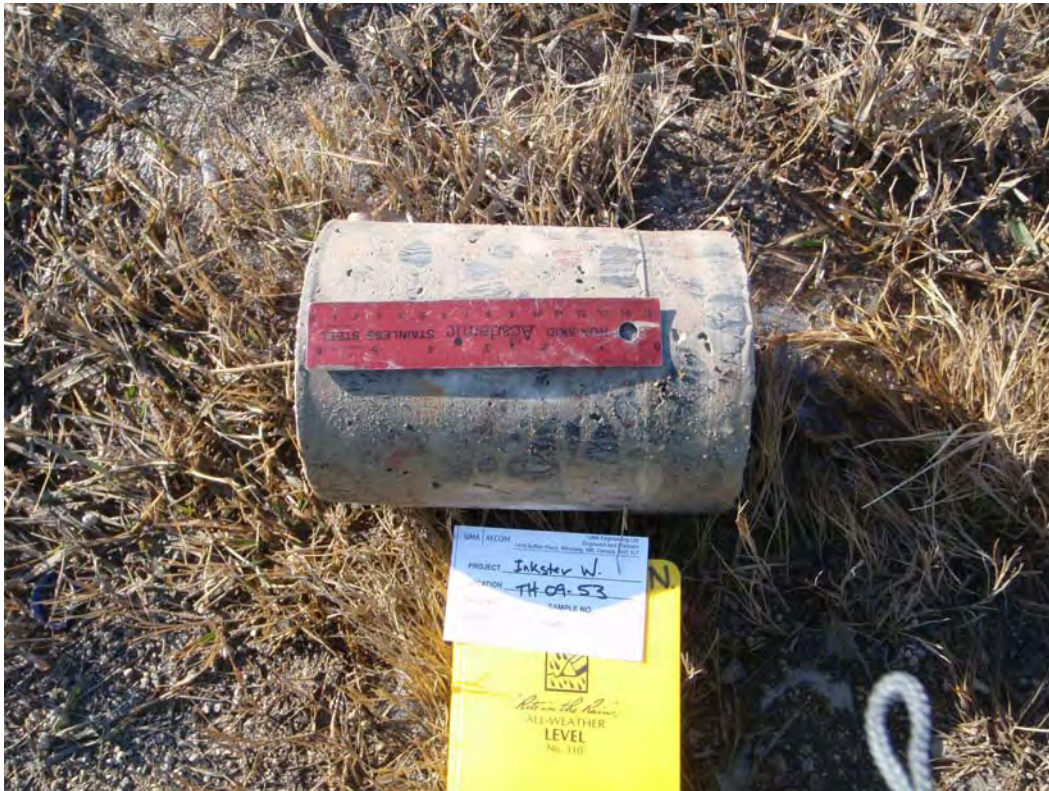
Photo 3: Core sample from TH-09-53
