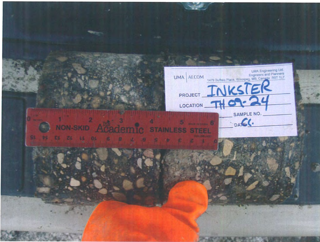
Photo 17: Core sample from TH-09-24
