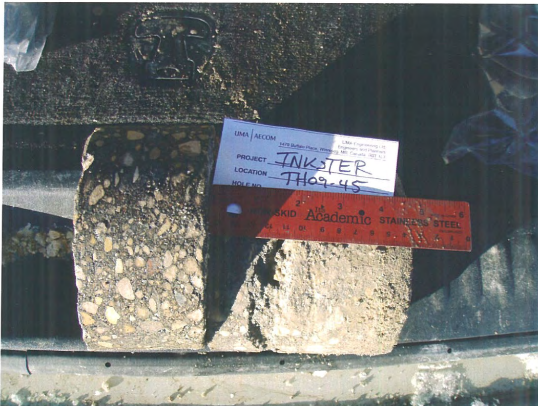
Photo 30: Core sample from TH-09-45
