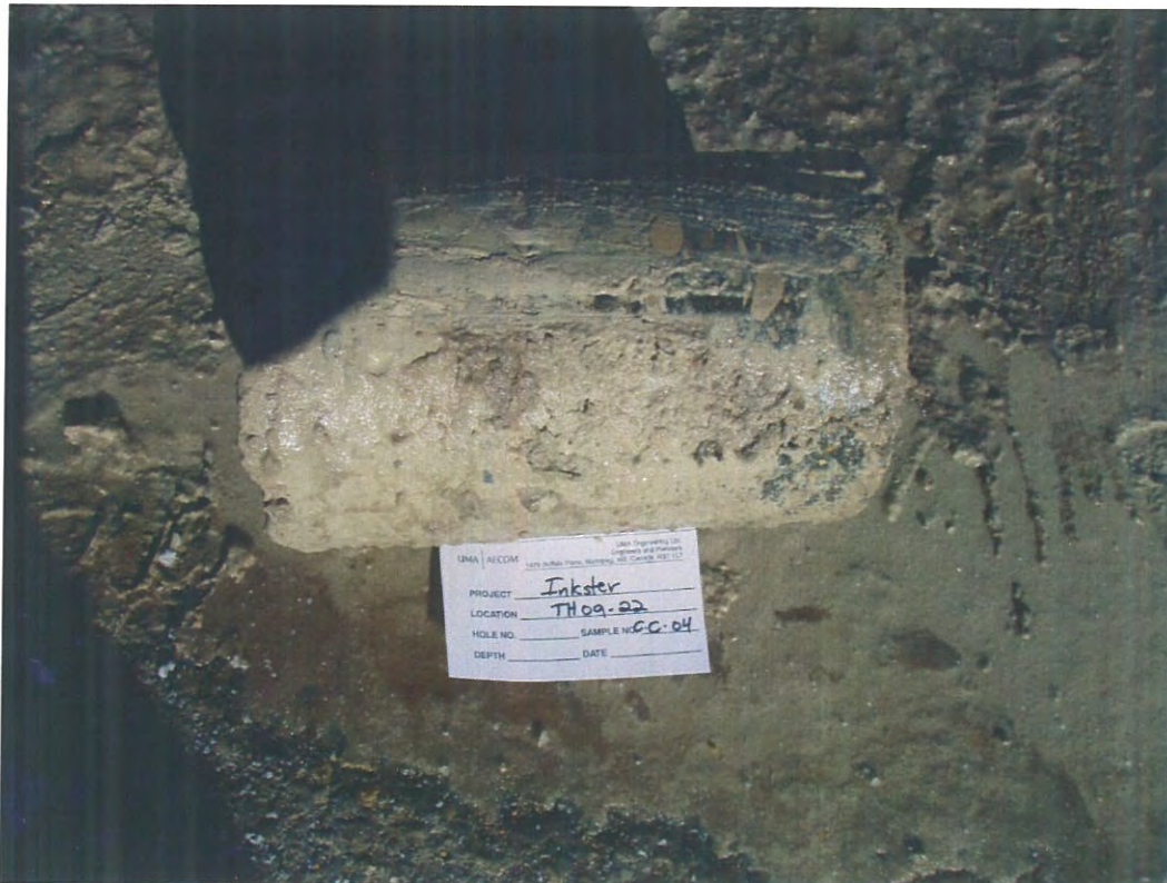
Photo 16: Core sample from TH-09-22
