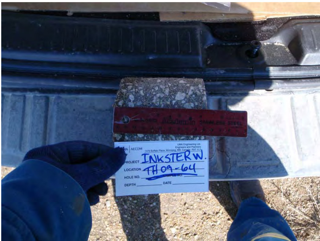
Photo 8: Core sample from TH-09-64
