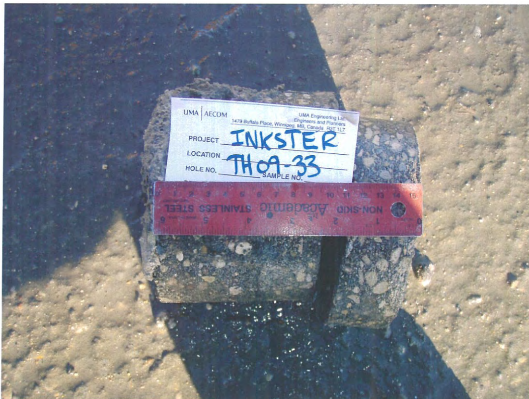
Photo 22: Core sample from TH-09-33
