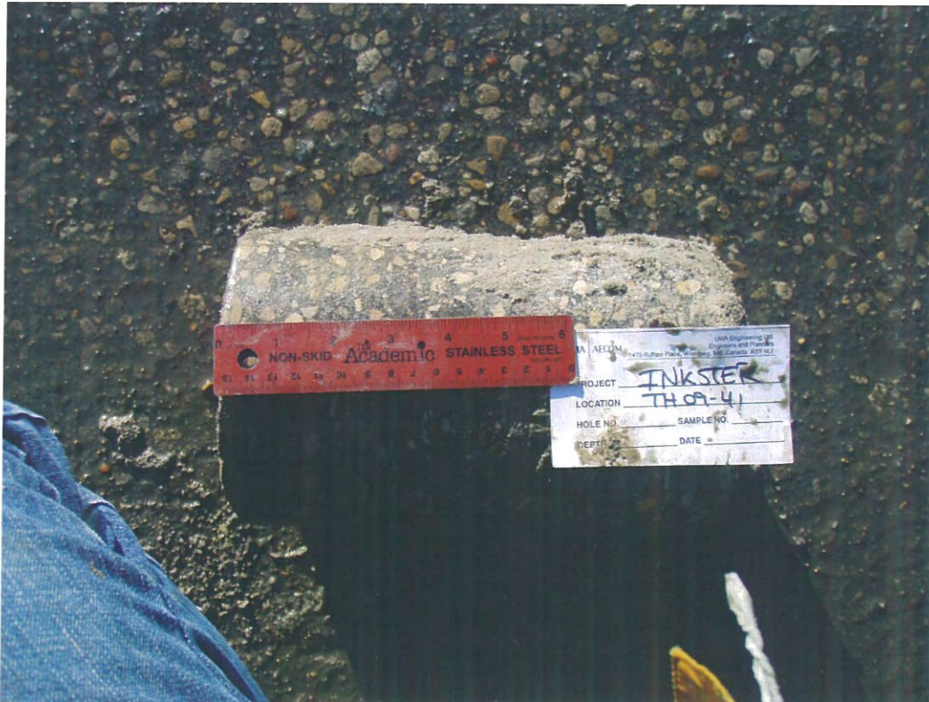
Photo 28: Core sample from TH-09-41
