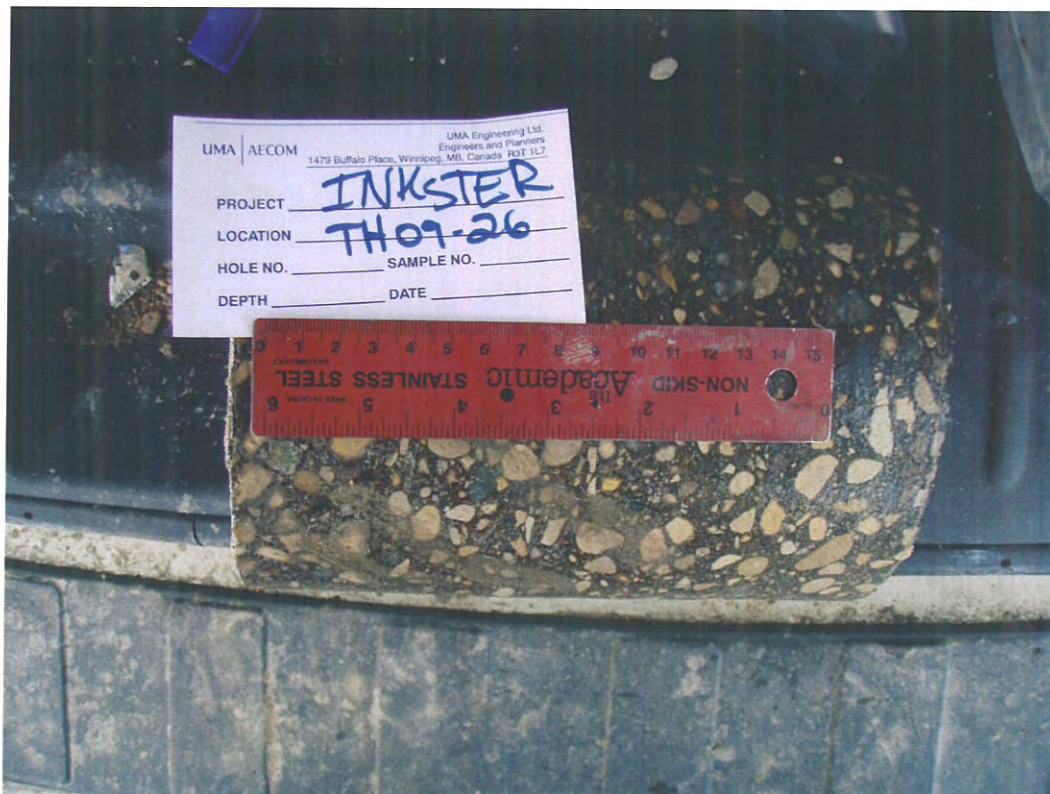
Photo 18: Core sample from TH-09-26
