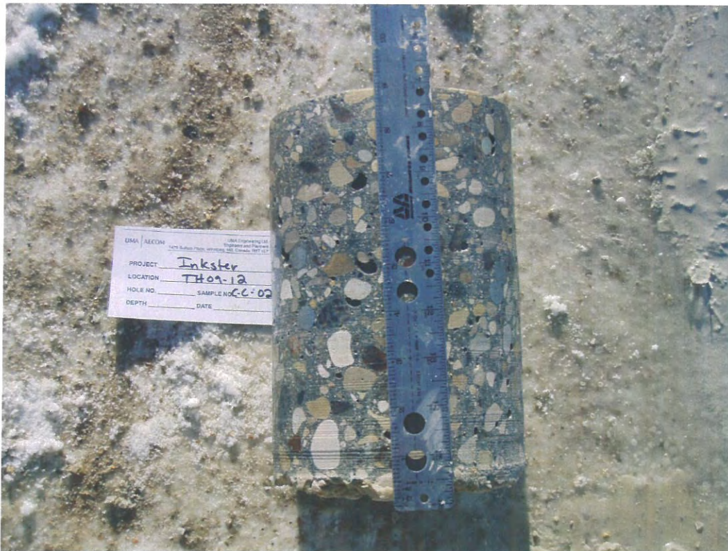
Photo 10: Core sample from TH-09-12
