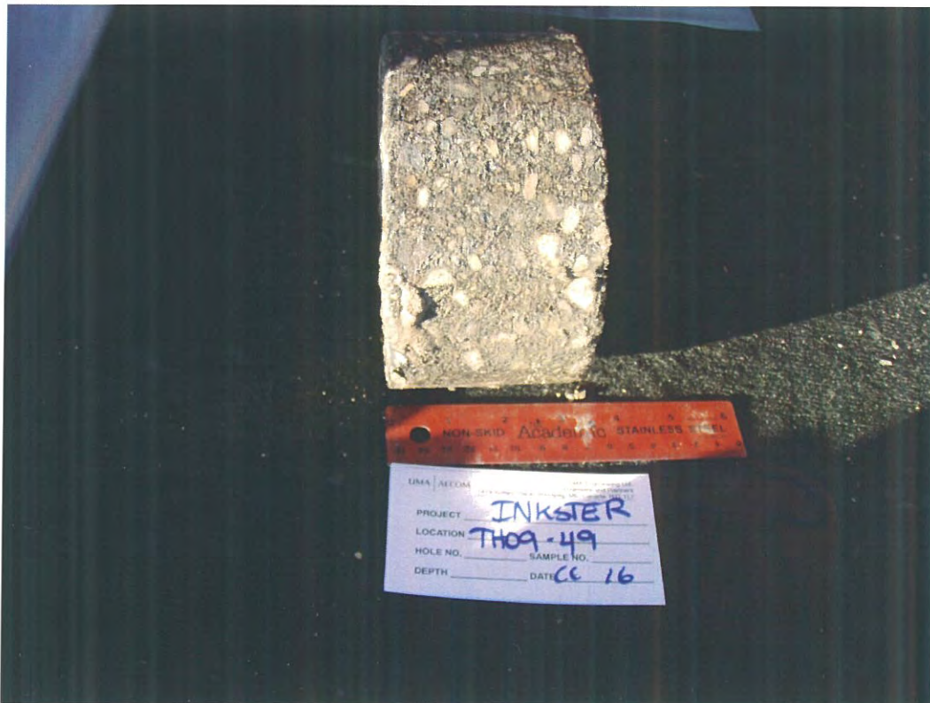
Photo 32: Core sample from TH-09-49
