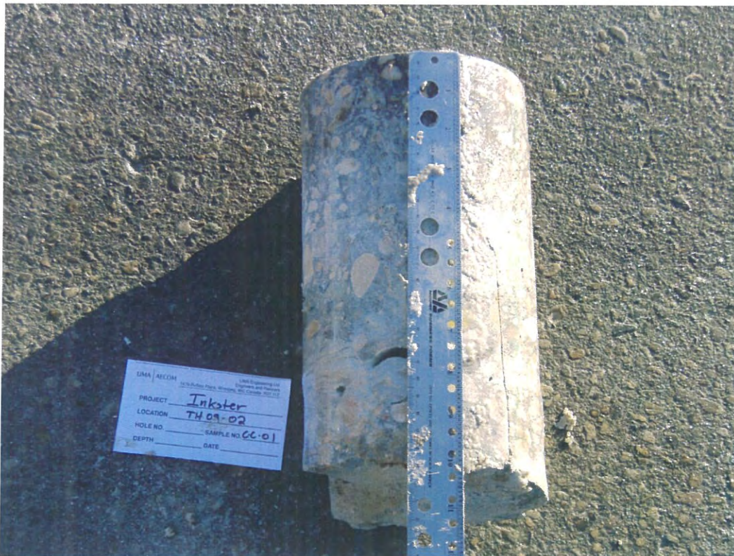
Photo 2: Core sample from TH-09-02
